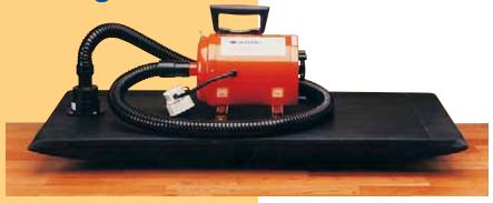
Primarily for seating wagons, the permanently installed type TB 400 theatre bearing has a capacity of 250 to 400kg. Each TB 400 combines with a dedicated 1hp blower unit (type AB 400), ensuring that eccentric loads can be accommodated without adjustment. A minimum of 3 combination TB/AB 400 units are required in each wagon to ensure stability, and two men can easily move 2000kg 'on air'.
