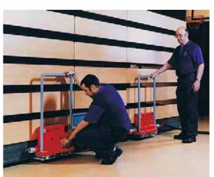
For lighter or more rigid loads, pairs of beams or planks are available, each incorporating two air bearings. These are located under the load using transit castors, and then connected to a mobile 3-phase blower pack located nearby. Operating the blowers inflates the air bearings and allows the load to be lifted prior to relocation.
