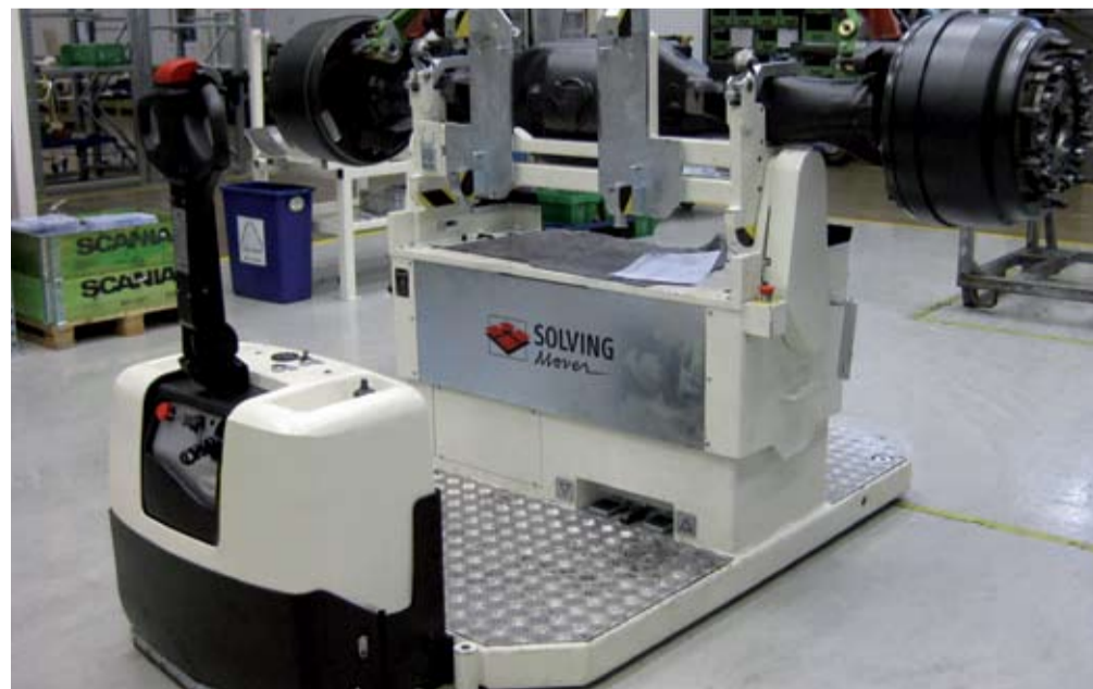
All axle types are assembled at Scania using five customised stand-on Movers from Solving.
