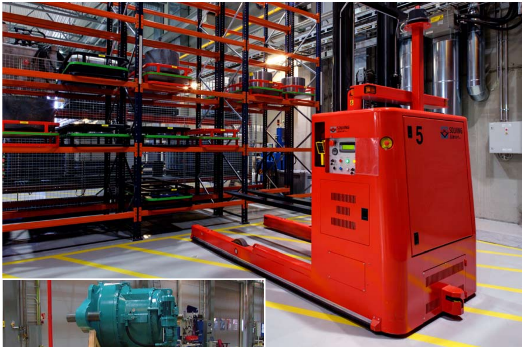
Air film Movers are installed to move heavy assembled gearboxes, whilst laser guided AGVs are used at the beginning of the production process for handling raw material.
