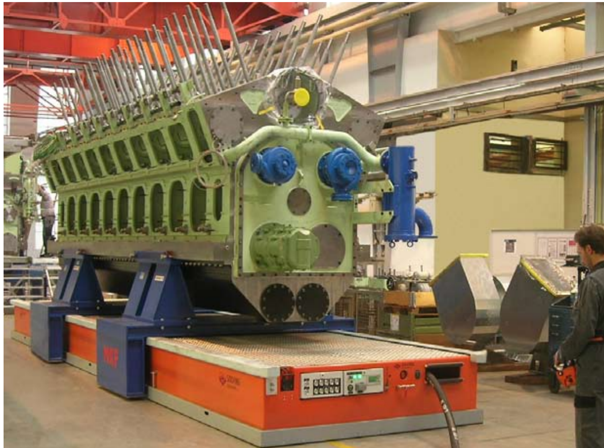
240-tonne diesel engines are assembled on an air film based Solving Mover.
