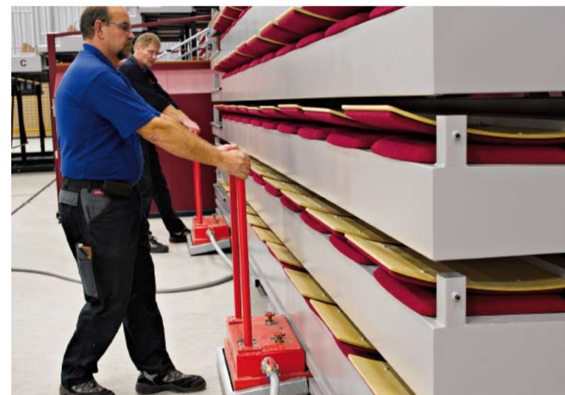
Air bearings facilitate the movement of seatings in multipurpose halls.
