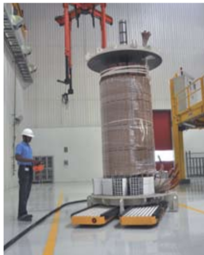
35-tonne windings are moved smoothly on a Solving air film Mover.
